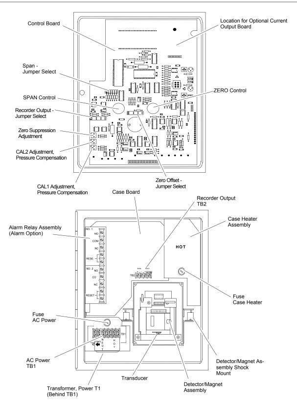
Figure 1-2. Model 755A Component and Adjustment Locations
